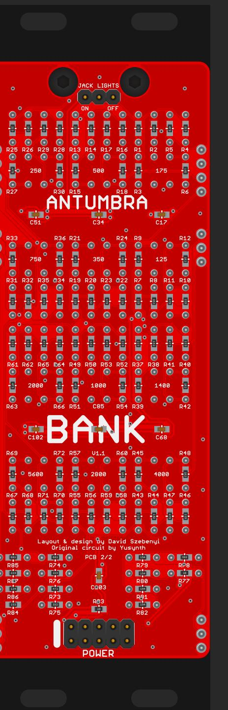
With the top header you can turn on or off the jack lights. Left position is on, right is off. Turning on the jack lights draw about 7mA more from the +12V rail.
